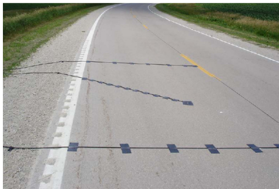
Figure 3.6 Roadtube Layout (From CTRE roadtube manual)
